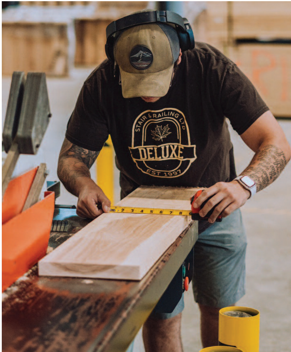
MEASURE TWICE, CUT ONCE - Daniel Sawers sizes a stair tread using a straight line rip saw. Deluxe Stair and Railing Ltd., located in Uxville, specializes in custom stair work. Submitted photo
